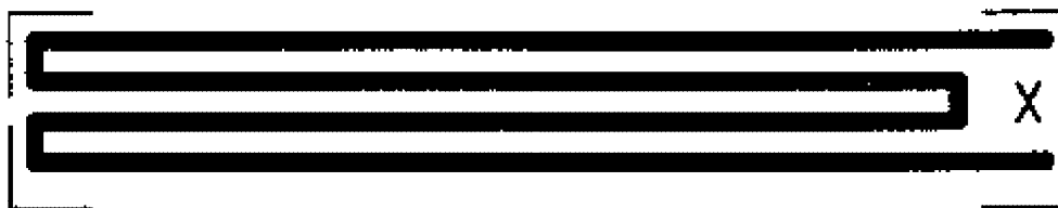
Figure 15: Example of test specimen layout for testing resistance to bending cycles
